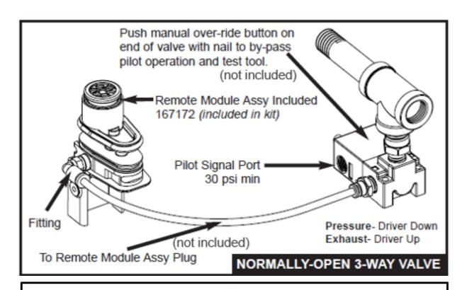
A 3-way normally open pilot operated valve is not included with this ETVA12-RF kit.
